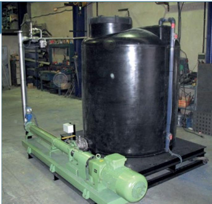
It is composed by: a water tank with cover and incoming and output piping for liquids, pump for the ...., pressure collector, shock absorbing for the blowing collector, interconnection set of valves and pipes between the water tank and the pump.
